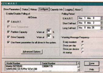
The great hard disk snoop EZ-SMART constantly watches for failure, and in this screen, can be instructed when and how to warn you.
